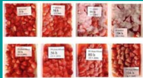
Strawberries in a conventional food container (upper row) and nano-silver container (lower row). (Test series and pictures: The Innovation Society Ltd.) Taken from Nanowerks, Feb 16, 2009
