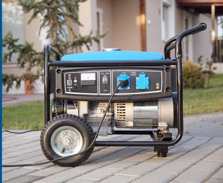
Portable generators are useful when temporary or remote electrical power is needed, like when the power goes out due to storms or you're out camping.
