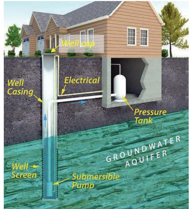
Wells can have a range of widths and depths. Typically, the deeper the well the better the water quality.
