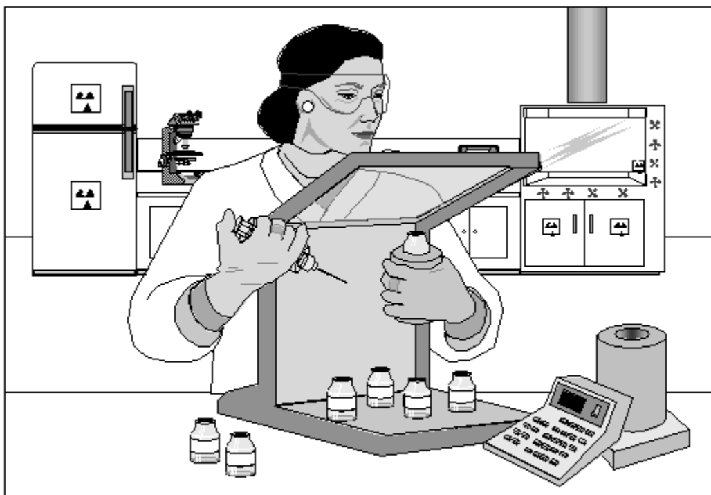
Figure 7: Use of Appropriate Shielding.
